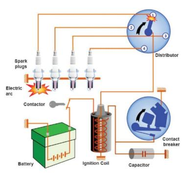
When the ignition switch is 'ON' the current flows from the battery through the primary winding and produces a magnetic field in the coil. When the contact points open the magnetic field 12 volts from the
